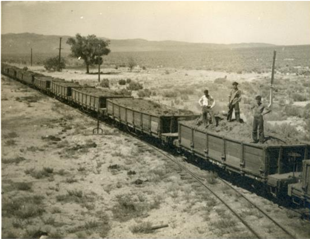
17, Three of the crew gloat atop our first full train out of Benton Station: left to right, Johnny Allingham, Pierce Clarke and Earl Williams. The sad state of these old cars, which had been inherited from older defunct narrow-gauge railroads, is seen in the bulging curve of their sides. They reminded us of the 1930s comic strip, Toonerville Trolley .
